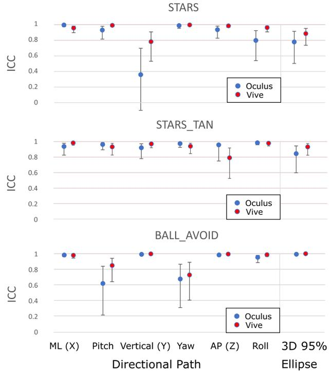
**Fig. 2.** Average Intraclass Correlation coefficients for 6 directional path measures (3 axes of translation and 3 axes of rotation) and a 3-dimensional 95% confidence ellipsoid for Oculus Rift (blue) and HTC Vive (red). Whiskers denote 95% confidence interval for the mean. (For interpretation of the references to colour in this figure legend, the reader is referred to the web version of this article.)
